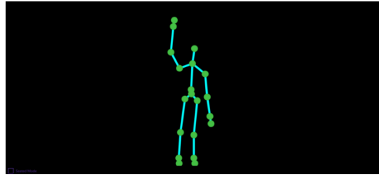
Figure 3(b): Gesture for the robot to turn right
