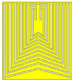
Fig. 15: M slot resonator-Adapted from Reference [49]
